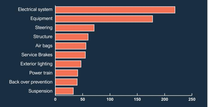
In 2023 the electrical system was responsible for the most recalls. This is common as it is a wide category that affects many aspects of the vehicles. NHTSA does not classify "software" as a component and so it does not list software as a "component at fault". However, we know that many of the electric system recalls will be attributed to software errors.
